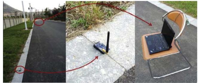
Fig. 8. Sensor deployment along a straight road. From left to right: the road, a normal sensor, and the sink.
